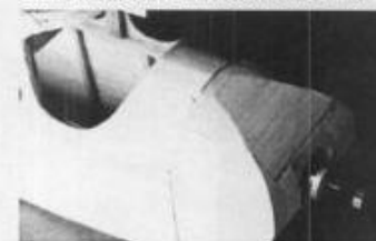
Cowl rough formed and glued to firewall.
