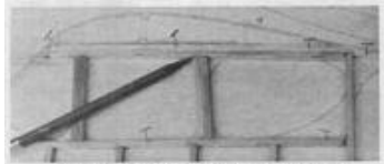
Laminate two sticks for cabin posts.
