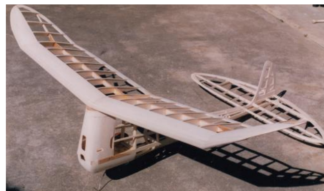
Framed up "Super Zomby" C Class April, 1942, "Air Trails". Built from Klarich Custom Kit won by Bill Britcher at Swan Hill. Model to use Edco Sky Devil .65 spark ignition engine. Original used retracting single wheel, Bill's version to use fixed single wheel.
