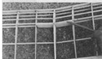
Wing halves joined with ply dihedral brace.
