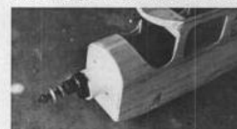
Motor and balsa tube in Astro mount. Add on the gear box for reduction drive version.
