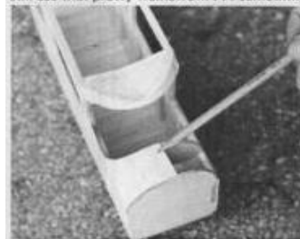
Curved portion of cowl after wet forming.
